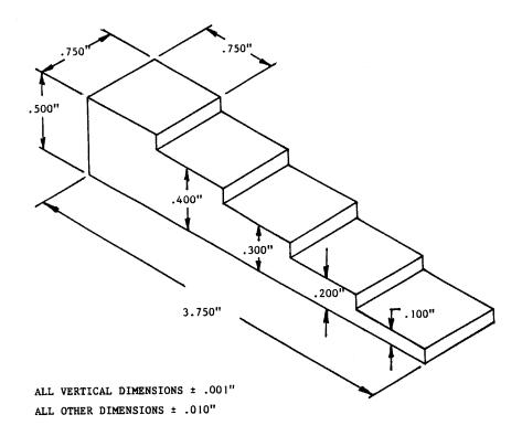
Note: The typical thickness reference block is supplied in Ni-plated C1018 steel and is also available in 7075 Aluminum and 304 Stainless Steel. A Metric version is also available in 2.5 mm steps in a thickness range of 2.5 mm to 12.5 mm.
