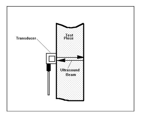
It is practically impossible to efficiently transmit ultrasound from the transducer to the object to be measured without the aid of a suitable coupling medium, usually referred to simply as couplant. Couplants frequently used for thickness gauging are water, oil, gel, glycerin, and propylene glycol. In practice, a small amount of couplant is applied between the transmitting face of the transducer and the test surface.
