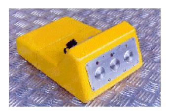
The **AMIGO** is one of a series of nondestructive testing ACFM (AC Field Measurement) instruments manufactured by **TSC Inspection Systems Ltd. (TSC)**, developed for the detection and sizing of defects in electrical conducting material. The new AMIGO represents a significant advance in topside inspection technology.
